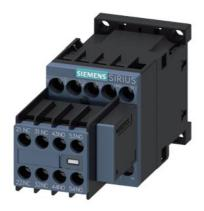
Power contactor, AC-3 9 A, 4 kW / 400 V 3 NO + 2 NC, 120 V AC 50 / 60 Hz, 3-pole, Size S00, screw terminal Varistor plugged on
