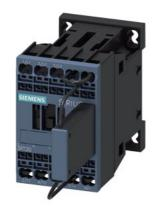
traction contactor, AC-3 16 A, 7.5 kW / 400 V 110 V DC 0.7-1.25\* US, with suppressor diode integrated 3-pole, size S00 spring-type terminal suitable for PLC outputs not expandable with auxiliary switch
