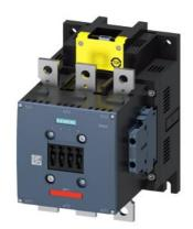
Power contactor, AC-3 265 A, 132 kW / 400 V Coil AC 50/60 Hz and DC 200-277 V x (0.8-1.1) F-SPS input 24 V DC 3-pole size S10 Auxiliary contacts 2 NO + 2 NC permanently mounted Main circuit: Busbar Control and auxiliary circuit: Screw terminal
