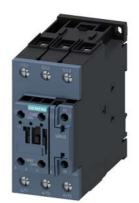
power contactor, AC-3 40 A, 18.5 kW / 400 V 1 NO + 1 NC, AC / DC 20-33 V, communication- capable, with varistor, 3-pole, Size S2, screw terminal
