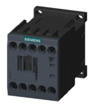
Contactor, AC-3, 7.5 KW / 400 V, 1 NC, 110 V AC, 50 / 60 Hz, 3-pole, Size S00 screw terminal
