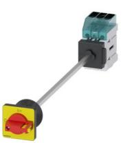
Load disconnector 3LD3, lu 40 A Main switch 3-pole Rated operating capacity at AC-23 A at 400 V 18.5 kW floor mounting Basic switch with door coupling Central hole mounting 22.5mm Toggle drive red / yellow 48x48 mm
