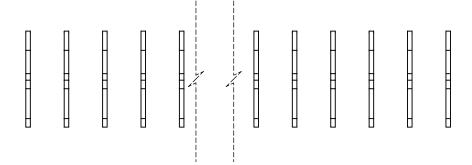
NOTE: CONTACTS ARE HELD IN A CARRIER FOR EASE OF ASSEMBLY
