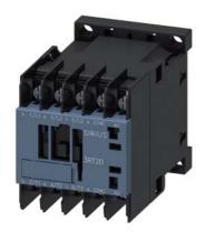
Power contactor, AC-3 7 A, 3 kW / 400 V 1 NC, 400 V AC, 50 Hz 400-440 V, 60 Hz, 3-pole, Size S00, ring cable lug connection
