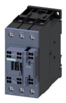
Power contactor, AC-3 65 A, 30 kW / 400 V 1 NO + 1 NC, 20-33 V AC/DC 3-pole, size S2 Spring-type terminals
