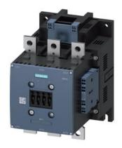
power contactor, AC-3 265 A, 132 kW / 400 V AC (50-60 Hz) / DC operation 220-240 V AC/DC auxiliary contacts 2 NO + 2 NC 3-pole, frame size S10 busbar connections drive: conventional spring-loaded terminal
