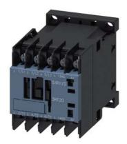
Power contactor, AC-3 16 A, 7.5 kW / 400 V 1 NO, 200 V AC, 50 Hz 200-220 V, 60Hz, 3-pole Size S00 ring cable lug connection
