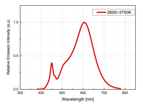
Fig 2. Radiant Pattern, T<sub>j</sub> = 25°C, I<sub>F</sub>=40mA
