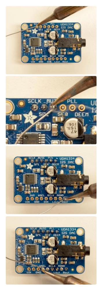
Solder each one of the pins into the board to make a secure connection
