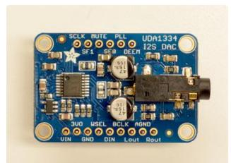
Make sure that all of the short parts of the header are sticking through the two sets of pads on either side of the board
