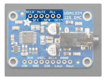
SCLK (Sys Clock) - Optional 27 MHz 'video mode' ssytem clock input - by default we generate the sysclock from the WS clock in 'audio mode' But the UDA can also take a oscillator input on this pin Mute - Setting this pin High will mute the output
