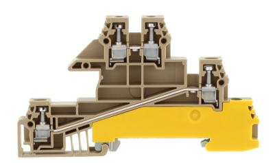
Three-wire installation terminal, Screw connection, Mounting type: Mounting rail TS 35/7.5, Rated cross-section: 2.5 mm², Width: 6 mm, Colour: Beige
