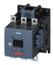
power contactor, AC-3 225 A, 110 kW / 400 V AC (50-60 Hz) / DC operation 110-127 V AC/DC auxiliary contacts 2 NO + 2 NC 3-pole, frame size S10 busbar connections drive: conventional screw terminal auxiliary switch block 2 NO + 2 NC lateral, left + right captive auxiliary switch block, DIN 50012
