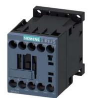
Coupling contactor relay, 2 NO + 2 NC, 110 V DC, 0.7 ... 1.25\* US, with integrated suppressor diode, Size S00, screw terminal suitable for PLC outputs
