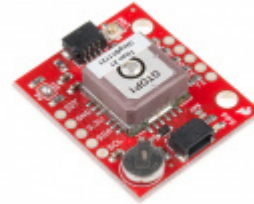
SparkFun GPS Breakout - XA1110 (Qwiic)
