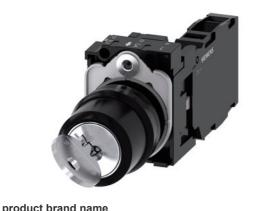
RONIS key-operated switch, 22 mm, round, plastic, lock number SB30, with 2 keys, 2 switch positions O-I, latching, 10:30h/13:30h, key removal O+I, with holder, 1 NO+1 NC, screw terminal, possible special locks: SB31, 421, 455, with laser labeling, upper case and lower case, always upper case at the beginning of the word
