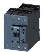
Power contactor, AC-3 50 A, 22 kW / 400 V 2 NO + 2 NC 175-280 V AC/DC varistor, 4-pole size S2 screw terminals 1 NO + 1 NC integrated
