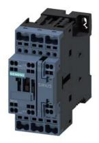
power contactor, AC-3 25 A, 11 kW / 400 V 1 NO + 1 NC, AC (50-60 Hz) DC operation 21-28 V AC/DC, 3-pole, Size S0, Spring-type terminal
