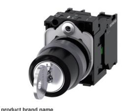
RONIS key-operated switch, 22 mm, round, plastic with metal front ring, lock number SB30, with 2 keys, 3 switch positions I-O-II, latching, actuating angle 2x45°, 10:30h/12h/13:30h, Key removal I+O+II, with holder, 1 NO, 1 NO, screw terminal, possible special locks: SB31, 421, 455, with laser labeling, upper case and lower case, always upper case at beginning of line
