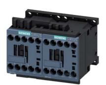
Reversing contactor assembly AC-3, 5.5 kW/400 V, 24 V DC 3-pole, Size S00 screw terminal electrical and mechanical interlock with integrated diode
