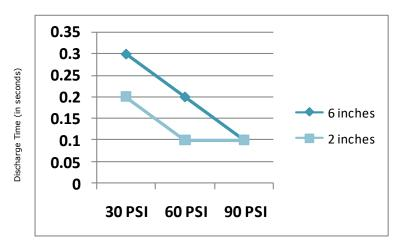
Offset voltage and discharge time per ANSI/ESD STM3.1 using a charged plate monitor with a 20pF,  $6^{\prime\prime}$  x  $6^{\prime\prime}$  plate. 1000 to 100 volts. Typical results.
