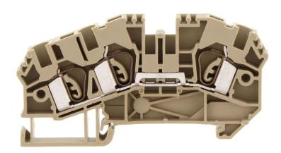
Ex feed-through terminal ATEX-certified, Tension-spring connection, Mounting type: Mounting rail TS 35/7.5, Rated cross-section: 4 mm², Width: 6.1 mm, Colour: Beige
