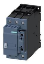
Capacitor contactor, AC-6b 50 kVAr, / 400 V 2 NC, 120 V AC, 60 Hz 3-pole, Size S2 screw terminal
