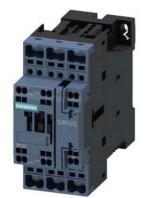
power contactor, AC-3 25 A, 11 kW / 400 V 1 NO + 1 NC, 125 V DC with integrated varistor 3-pole, size S0, spring-type terminal suitable for PLC outputs not expandable with auxiliary switch
