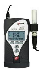
Battery powered datalogger for external CO2 probe up to 10 000ppm and inputs for connecting up to three temperature and/or humidity probes. Multilogger can be installed permanently to Ethernet network or work as portable device.
