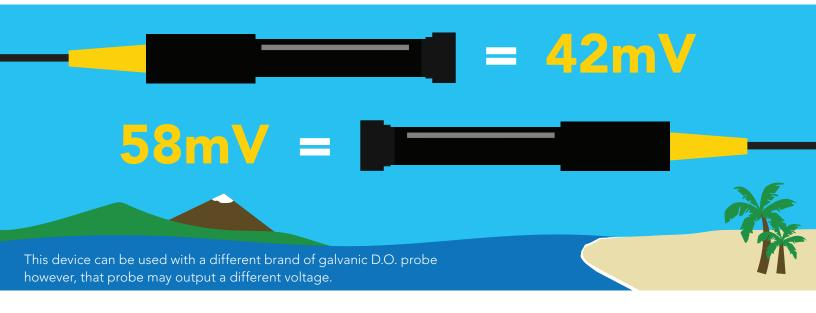
The analog voltage coming off pin A is the voltage from the probe + an 11x gain. This means the analog voltage read on pin A is the voltage from the probe x11.
