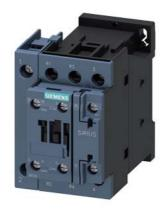
Power contactor, AC-3 25 A, 11 kW / 400 V 2 NO + 2 NC 230 V AC, 50 Hz 4-pole size S0 screw terminals 1 NO + 1 NC integrated
