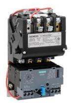
Non-reversing motor starter Size 00 Three phase full voltage Solid-state overload relay OLRelay amp range 0.75-3.4A 190-220/220-240V 50/60HZ coil Combination type No enclosure
