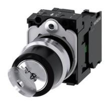
RONIS key-operated switch, 22 mm, round, metal, shiny, lock number SB30, with 2 keys, 2 switch positions O-I, latching, actuating angle 90°, 10:30h/13:30h, key removal O+I, with holder, 1 NO, screw terminal, possible special locks: SB31, 421, 455, upper case and lower case, always upper case at beginning of line
