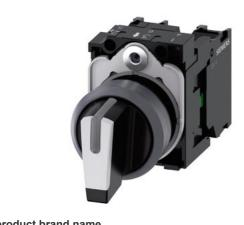
Selector switch, illuminable, 22 mm, round, plastic with metal front ring, white, selector switch, short, 3 switch positions I>O<II, momentary contact type, actuating angle 2x45°, 10:30h/12h/13:30h, with holder, 1 NO, 1 NO, screw terminal, with laser labeling, upper case and lower case, always upper case at beginning of line
