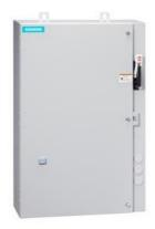
Non-reversing motor starter, Size 3, Three phase full voltage, Solid-state overload relay, OLR amp range 25-100A, 110V 50Hz / 120V 60Hz coil, Combination type, 100A non-fusible disconnect, Encl NEMA type 4X 304 S-Steel, Water/dust tight noncorrosive, Standard width enclosure
