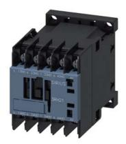
Contactor relay, 4 NO, 200 V AC, 50 Hz, 200  $\mathinner{\ldotp\ldotp}$  220 V, 60 Hz, Size S00, ring cable lug connection
