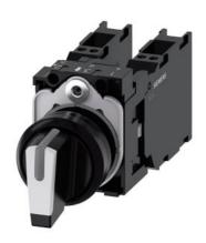
Selector switch, illuminable, 22 mm, round, plastic, white, selector switch, short, 3 switch positions I-O-II, latching, 10:30h/12h/13:30h, with holder, 2x1NO+1NC, Spring-type terminal
