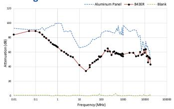
Test performed with a two-coat thickness.
