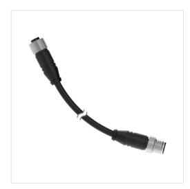
Cordset A-Code M12 to A-Code M12 Double Ended 17-Pin Straight Female; 17-Pin Straight Male Connectors with Shield 9.14 m (29.98 ft) in Length Black PVC Jacket, Nickel Plated Brass Nut
