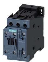
Power contactor, AC-3 38 A, 18.5 kW / 400 V 1 NO + 1 NC, 24 V DC communication-capable, 3-pole Size S0, screw terminals
