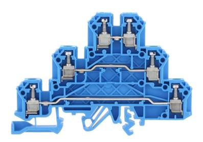
Three-level initiator terminal | Multi-wire terminal, Screw connection, Mounting type:Mounting rail TS 35/7.5 and TS 32, Rated cross-section: 2.5 mm², Width: 5 mm, Colour: Blue
