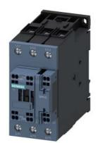
Traction contactor, AC-3 65 A, 30 kW / 400 V 1 NO + 1 NC 72 V DC, 0.7-1.25\* Us with varistor 3-pole, size S2 Spring-type terminals
