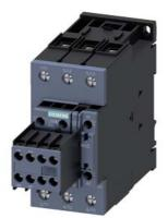
power contactor, AC-3 51 A, 22 kW / 400 V 2 NO + 2 NC, 220 V AC, 50 Hz / 240 V, 60 Hz, 3-pole, size S2, screw terminal
