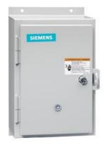
Reversing motor starter, Size 1, Three phase full voltage, Solid-state overload relay, OLR amp range 10-40A, 208VAC 60Hz coil, Non-combination type, Enclosure type 12, Dust/drip proof for indoors, Standard width enclosure
