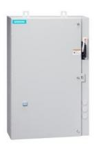
Non-reversing motor starter Size 1 3/4 Three phase full voltage Solid-state overload relay OLRelay amp range 10-40a 24VAC 50-60HZ coil Combination type 40AMP circuit breaker Enclosure NEMA type 4/12 Water/dust tight for outdoors Extra-wide enclosure
