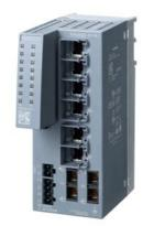
SCALANCE XC106-2, Unmanaged IE switch, 6x 10/100 Mbit/s RJ45 ports, 2x 100 Mbit/s Multimode LC, LED diagnostics, error-signaling contact with set pushbutton, redundant power supply Manual available as a download .
