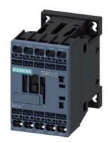
Power contactor, AC-3 16 A, 7.5 kW / 400 V 1 NC, 48 V DC 3-pole, Size S00 Spring-type terminals
