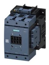
power contactor, AC-3 115 A, 55 kW / 400 V AC (50-60 Hz) / DC operation 96-127 V AC/DC auxiliary contacts 2 NO + 2 NC 3-pole, frame size S6 with box terminals drive: electronic with PLC interface 24 V DC spring-loaded terminal
