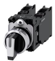
Selector switch, illuminable, 22 mm, round, metal, shiny, white, selector switch, short, 3 switch positions I>O<II, momentary contact type, actuating angle  $2x45^{\circ}$ , 10:30h/12h/13:30h, with holder, 2 x 1 NO+1 NC, spring-type terminal, Z=20-unit packaging
