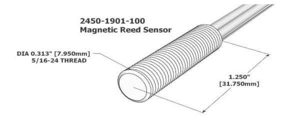
All measurements are in Inches [millimeters]
