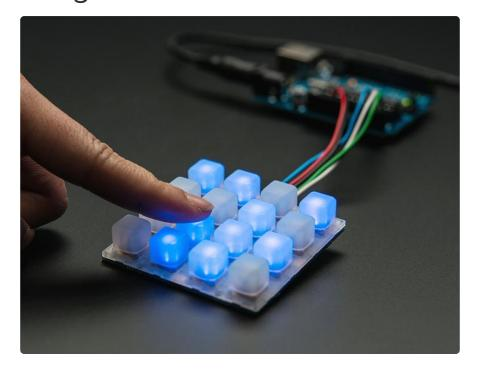
As shown here, Trellis is just an LED/keypad controller. You still need an Arduino or similar to do the work of reading the keypad data and then signifying when to light LEDs.
