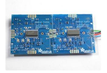
Solder two blobs of solder on two adjacent finger pads.
