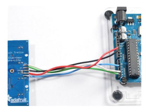
Now open up the Arduino IDE and open up the File->Examples->Adafruit\_Trellis->TrellisTest example sketch and upload it to your Arduino
