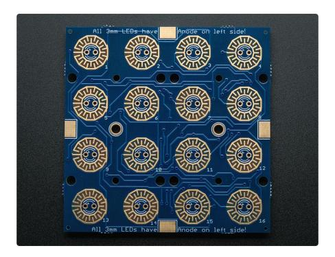
The Trellis PCB is specially made to match the Adafruit 4x4 elastomer keypad. Each Trellis PCB has 4x4 pads and 4x4 matching spots for 3mm LEDs. The circuitry onboard handles the background key-presses and LED lighting for the 4x4 tile. However, it does not have any microcontroller or other 'brains' - an Arduino (or similar microcontroller) is required to control the Trellis to read the keypress data and let it know when to light up LEDs as desired.
