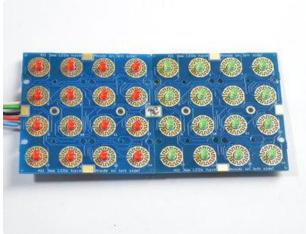
You can add a little more mechanical stability by soldering the large front tabs as well
