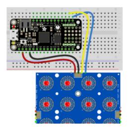
Board 3V to Trellis 5V/VCC Board GND to Trellis GND Board SCL to Trellis SCL Board SDA to Trellis SDA
