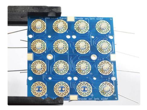
LEDs have polarity so they have to be installed the right way or they won't work! There's a little + symbol on the left hand LED pads, thats the anode/positive pin. LEDs have a longer leg on the + pin so make sure that pin goes into the + hole.
