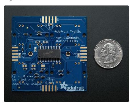
Each tile has an I2C-controlled LED sequencer and keypad reader already on it. The chip can control all 16 LEDs individually, turning them on or off. It cannot do grayscale or dimming. The same chip also reads any keypresses made with the rubber keypad. The connections are 'diode multiplexed' so you do not have to worry about "ghosting"
