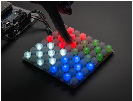
Trellis is an open source backlight keypad driver system. It is easy to use, works with any 3mm LEDs and eight tiles can be tiled together on a shared I2C bus.
