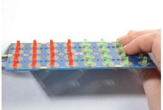
Check that the panels are aligned by looking from the side, gently bend/reheat until they are nice and straight
