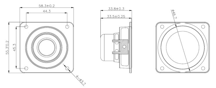
Note: Recommended speaker baffle opening is 53.5mm. Always test-fit prior to closing mechanical design. Please maintain at least 6mm distance between top of frame and next surface.
