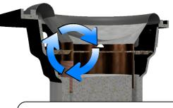
Air is forced into the magnetic loop on both sides of the voice coil for improved heat dissipation
